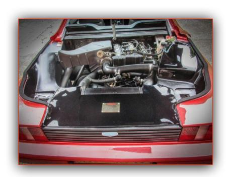
The engine is a turbo-charged 2 Litre, four-cylinder Cosworth unit similar to the one fitted to the famous Sierra Cosworth. It develops 204 bhp at 6000 rpm and 200 lb ft of torque at 4500 rpm. Unlike any other mid-engined Supercar, the Solo's engine is mounted not only north-south but also asymmetrically in both vertical and horizontal planes in order to make room for the 4WD transmission. This was to avoidt adding length to the wheelbase.
